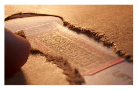
Fig. 5. Angled Light Attack on PINTAB Mailer (Nominet UK, Jun 2005), brown envelope mask used to reduce glare for purposes of photography
