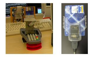
This device records ISO 7816 transactions, and we monitored communications between real EMV terminals and cards. Also, we wrote a PC implementation of the core terminal software
