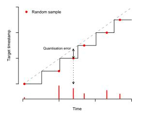
Only the samples made near clock edges contribute to the accuracy of the skew measurement
