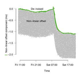
Measure clock offset of candidate machine(s) Remove constant skew from offset Remove noise Differentiate and negate
